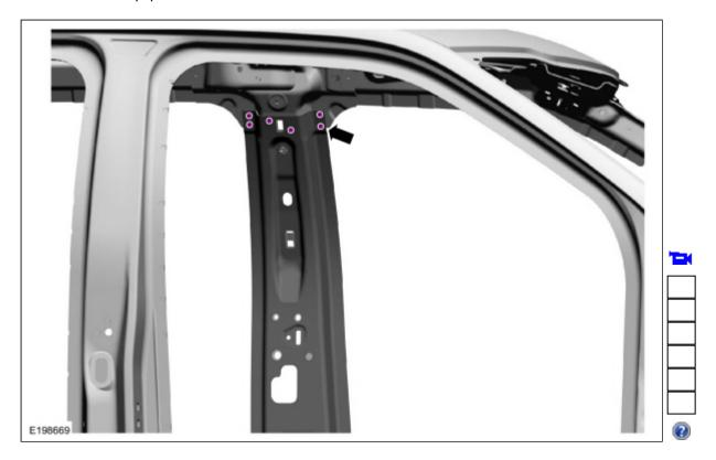
7. Remove and discard the <u>FDS</u> fasteners.
