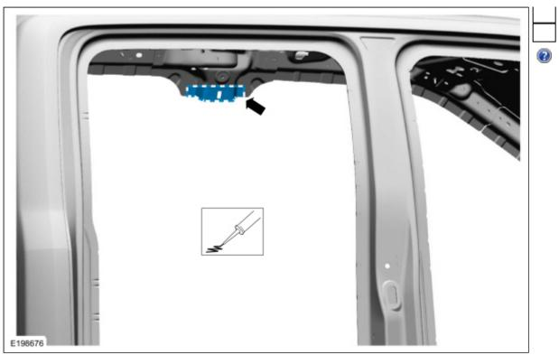
Apply adhesive. Material: Metal Bonding Adhesive / TA-1, TA-1-B, 3M<sup>™</sup> 08115, LORD Fusor® 108B
