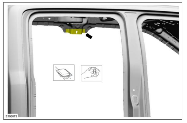
3. Sand using 80 grit sand paper to remove e-coat and clean the B-pillar service panel lower mating surface.
