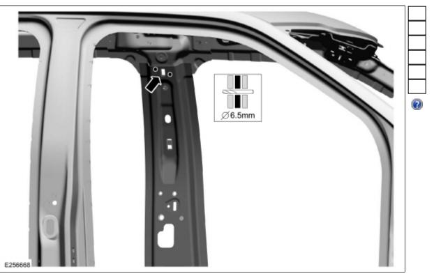
9. NOTE: Do not install <u>SPR</u> fasteners directly in old <u>SPR</u> fastener location. <u>SPR</u> fasteners must be installed adjacent to the original location matching original quantity.
