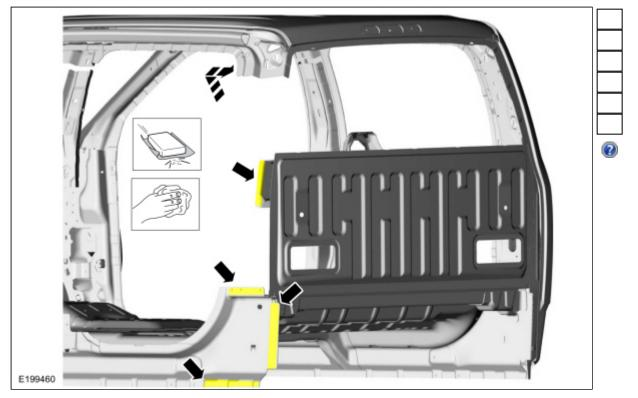
2. Sand using 80 grit sand paper to remove old adhesive and e-coat and clean.
