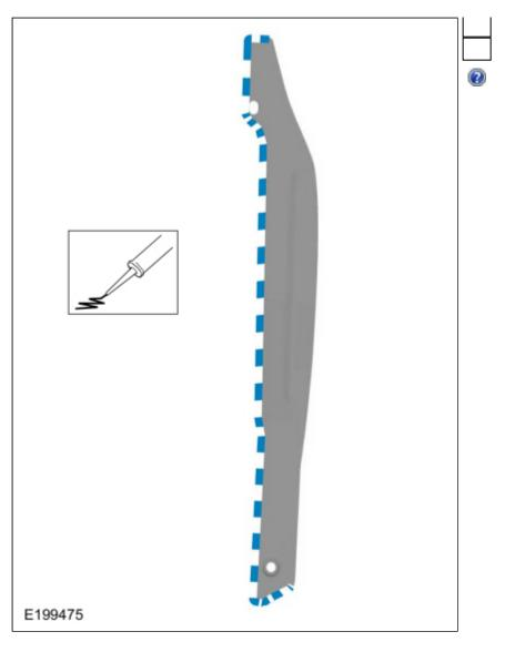
27. Install the cab back filler panel and clamp in position. Use the General Equipment: Locking Pliers
