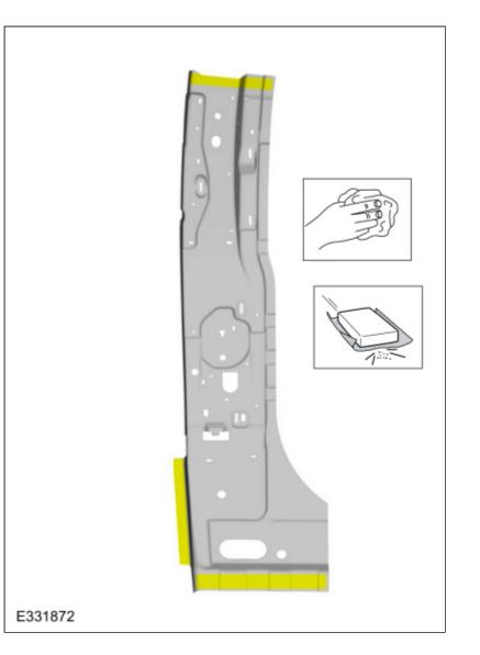
3. Apply adhesive to the service part mating surfaces. *Material*: Metal Bonding Adhesive / TA-1, TA-1-B, 3M<sup>™</sup> 08115, LORD Fusor® 108B
