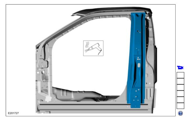
25. Remove and discard the <u>FDS</u> fasteners. Use the General Equipment: Polydrive Bit Socket
