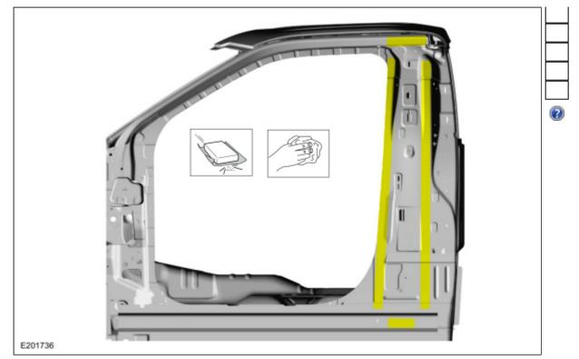
Apply adhesive. Material: Metal Bonding Adhesive / TA-1, TA-1-B, 3M<sup>™</sup> 08115, LORD Fusor® 108B
