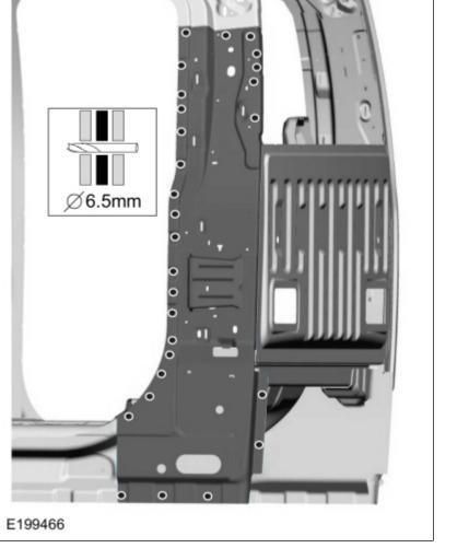
6. NOTE: <u>SPR</u> fasteners may not be placed directly over original <u>SPR</u> location. They must be placed adjacent to original location matching original quantity. Install the fasteners.
