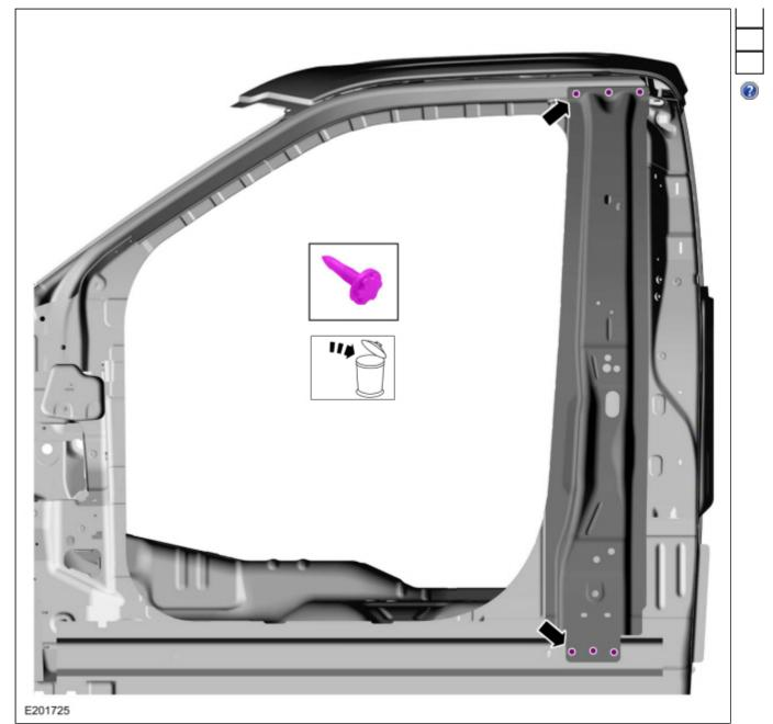
23. Remove the <u>SPR</u> fasteners.
