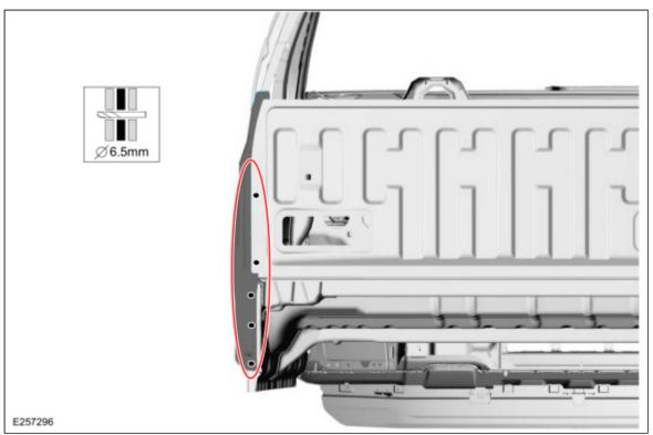
29. NOTE: <u>SPR</u> fasteners may not be placed directly over original <u>SPR</u> location. They must be placed adjacent to original location matching original quantity.
