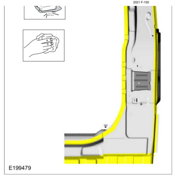
17. Sand the service panel mating surfaces using 80 grit sand paper to remove e-coat and clean.
