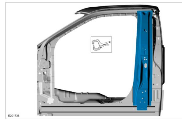
10. Drill 6.5 mm holes for blind rivet fastener installation. Use the General Equipment: 6.5 mm Drill Bit
