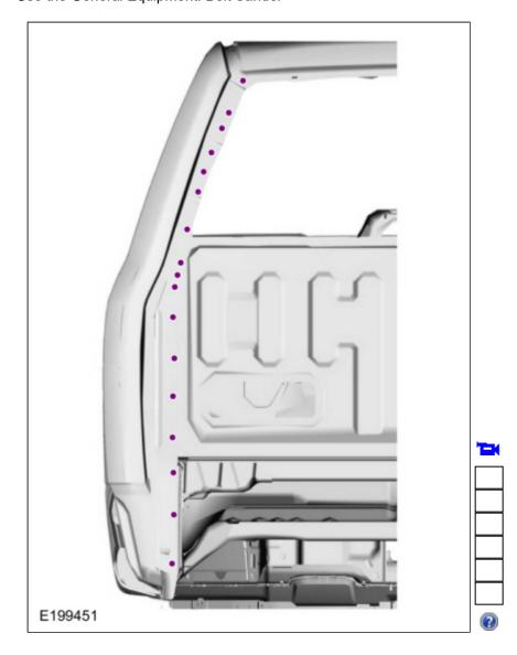
17. Remove the <u>SPR</u> fasteners.
