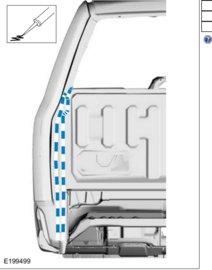
35. Refinish the entire repair using a Ford approved paint system and typical refinishing techniques.
