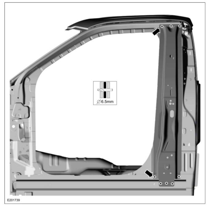
11. Install blind rivet fasteners.
