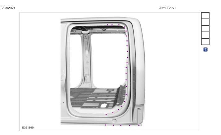
18. NOTICE: Body side sectioning is prohibited within 50mm of door hinge, door striker and restraints anchoring points.
