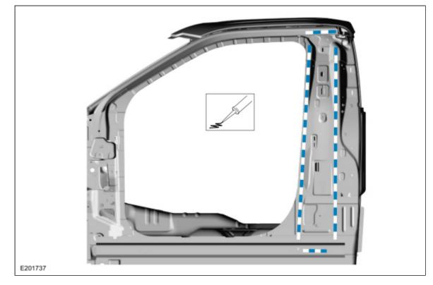
9. Install the C-pillar reinforcement and clamp in position. Use the General Equipment: Locking Pliers
