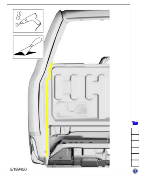
16. Remove the <u>SPR</u> fasteners.
