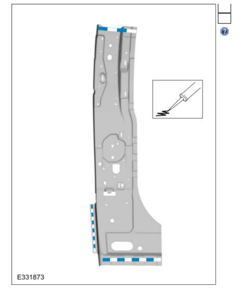
4. Install the C-pillar reinforcement and clamp in position. Use the General Equipment: Locking Pliers
