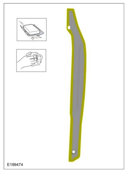
26. Apply adhesive as indicated to the cab back filler panel mating surface. *Material*: Metal Bonding Adhesive / TA-1, TA-1-B, 3M<sup>™</sup> 08115, LORD Fusor® 108B
