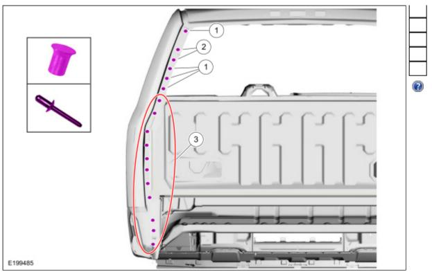
30. Metal finish all sectioning seams using typical aluminum metal finishing techniques and a fiber-based filler. Refer to: <u>Special Repair Considerations for Aluminum Repairs</u> (501-25 Body Repairs - General Information, Description and Operation).
