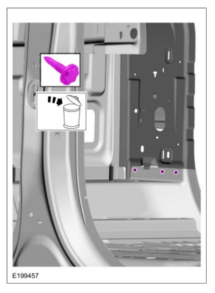
26. Remove the fasteners.
