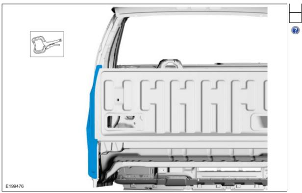
28. Drill for fasteners. Use the General Equipment: 6.5 mm Drill Bit
