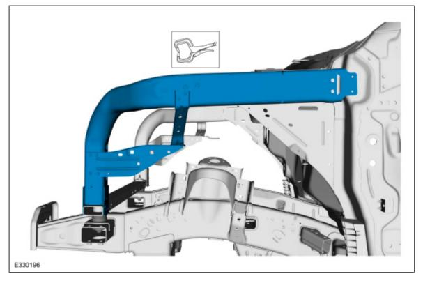
5. Install the bolts. *Torque*: 22 lb.ft (30 Nm)
