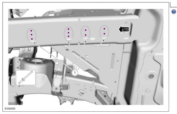
12. Install the bolts. *Torque*: 22 lb.ft (30 Nm)
