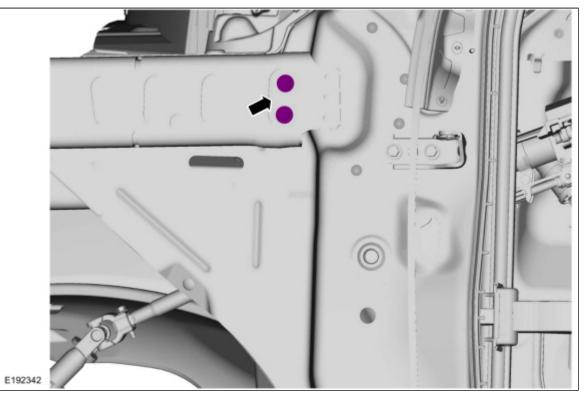
15. Remove the <u>SPR</u> fasteners. Use the General Equipment: Self-Piercing Rivet (SPR) Remover/Installer Use the General Equipment: Belt Sander
