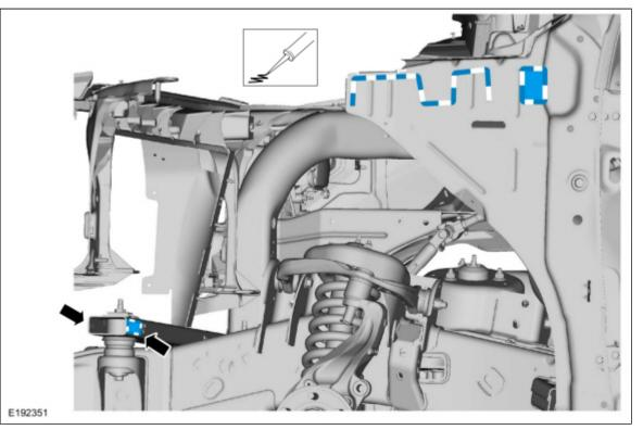
4. Install, properly position and clamp the fender apron panel reinforcement assembly. Use the General Equipment: Locking Pliers
