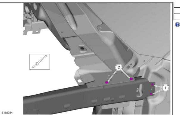
8. Drill rivet holes as indicated. Use the General Equipment: 6.5 mm Drill Bit
