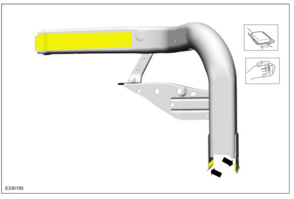
3. Apply adhesive. *Material*: Metal Bonding Adhesive / TA-1, TA-1-B, 3M<sup>™</sup> 08115, LORD Fusor® 108B
