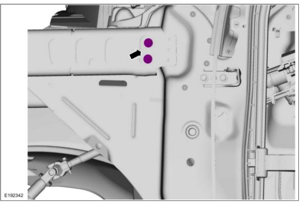
6. Drill rivet holes as indicated. Use the General Equipment: 6.5 mm Drill Bit
