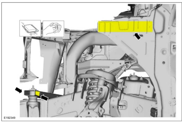
2. Sand to remove e-coat in the mating surface area only using 80 grit sandpaper and clean.
