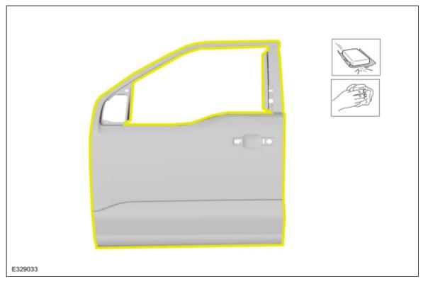
4. Apply adhesive. *Material*: Metal Bonding Adhesive / TA-1, TA-1-B, 3M<sup>™</sup> 08115, LORD Fusor® 108B
