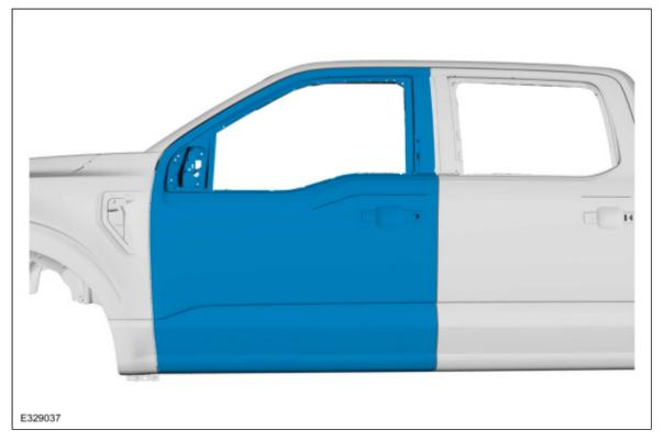
7. Check the door panel for proper fit and alignment.
