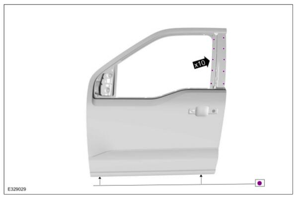
11. Carefully grind the **outer layer only** of the door skin hem flange as indicated. Use the General Equipment: Grinder
