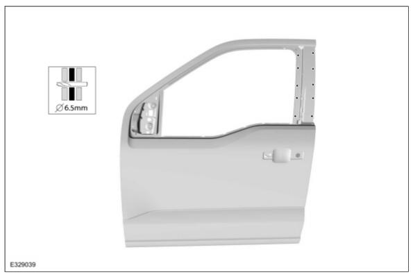
10. **NOTE**: <u>SPR</u> fasteners may not be placed directly over original <u>SPR</u> location. They must be placed adjacent to original location matching original quantity. **NOTE**: Blind rivet or solid rivet fasteners may be used in place of <u>SPR</u> fasteners after enlarging holes to 6.5 mm.
