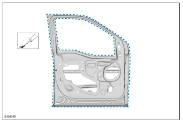
5. NOTICE: To prevent work-hardening of the metal do not use the hammer and dolly method for closing the hem flange. A hem flanging tool designed to work with aluminum is the preferred method.
