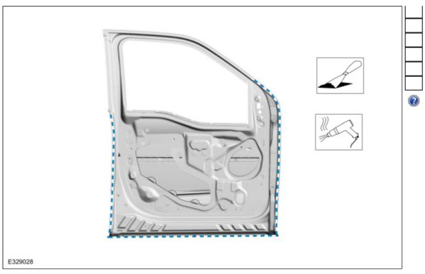
Remove the <u>SPR</u> fasteners as indicated.
