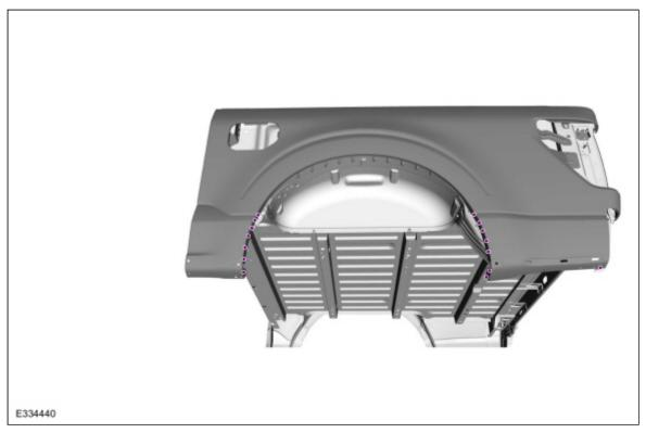
12. Remove the <u>SPR</u> fasteners.
