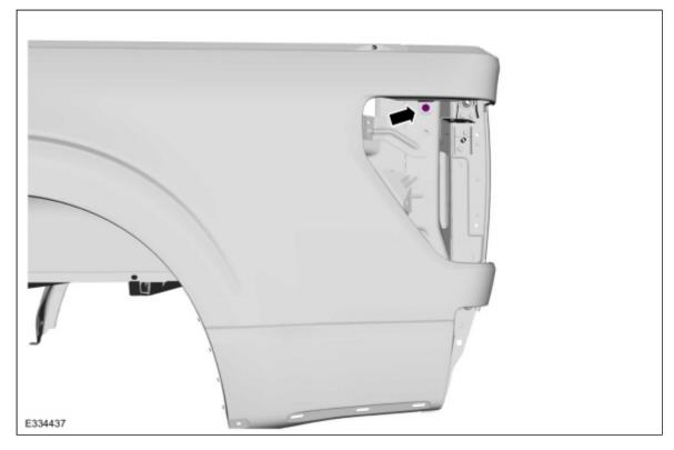
8. Remove the <u>SPR</u> fasteners.
