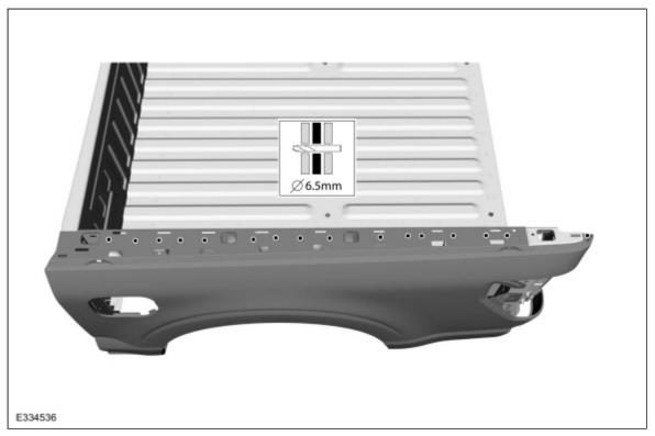
16. **NOTE:** Blind rivets, solid rivet fasteners or aluminum <u>MIG</u> plug welds may be used in place of <u>SPR</u> fasteners after enlarging holes to 6.5 mm. Install fasteners.
