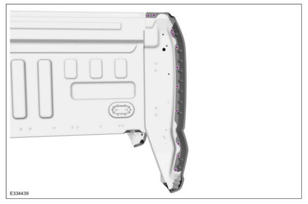
11. Remove the <u>SPR</u> fasteners.
