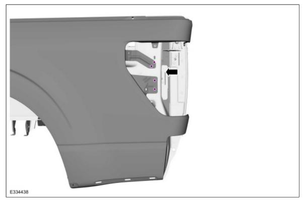
Remove the <u>SPR</u> fasteners.
