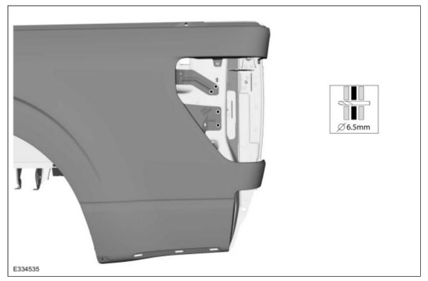
10. **NOTE:** Blind rivets, solid rivet fasteners or aluminum <u>MIG</u> plug welds may be used in place of <u>SPR</u> fasteners after enlarging holes to 6.5 mm. Install fasteners.
