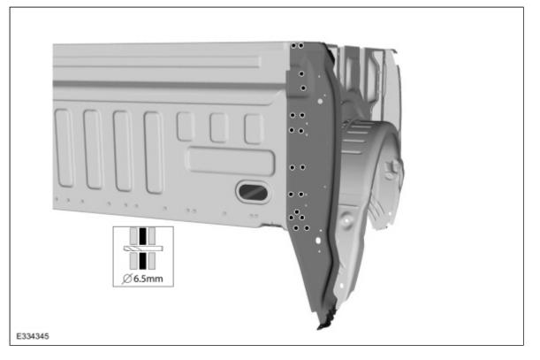
12. NOTE: Blind rivets, solid rivet fasteners or aluminum <u>MIG</u> plug welds may be used in place of <u>SPR</u> fasteners after enlarging holes to 6.5 mm.
