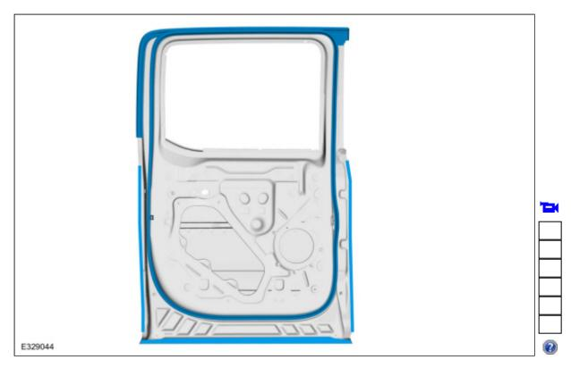
Remove the seam sealer from the door hem flange.
