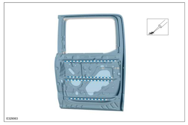
16. Refinish the door shell flange using a Ford approved paint system and typical refinishing techniques.
