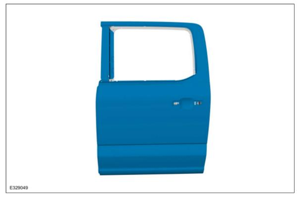
Remove the remaining portion of the door outer panel hem flange. Use the General Equipment: Knife Use the General Equipment: Hot Air Gun
