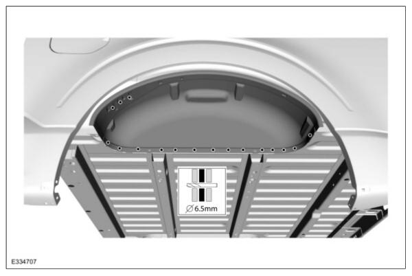
3. **NOTE**: <u>SPR</u> fasteners may not be placed directly over original <u>SPR</u> location. They must be placed adjacent to original location matching original quantity. **NOTE**: Blind or solid rivet fasteners may be used in place of <u>SPR</u> fasteners after enlarging holes to 6.5 mm.
