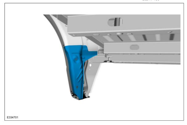
8. Remove the inner to outer wheelhouse <u>SPR</u> fasteners.
