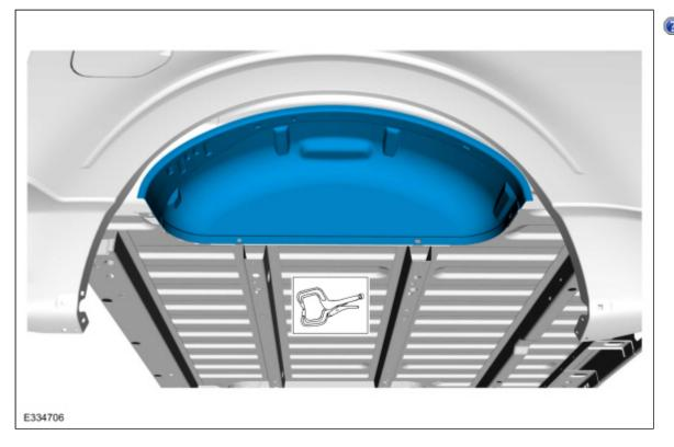
2. **NOTE**: Blind or solid rivet fasteners may be used in place of <u>SPR</u> fasteners after enlarging holes to 6.5 mm.
