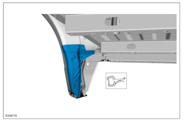
14. Drill for fastener installation.
