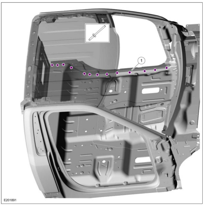
Install the C-pillar reinforcement. Refer to: <u>C-Pillar Reinforcement</u> (501-29 Side Panel Sheet Metal Repairs, Removal and Installation).
