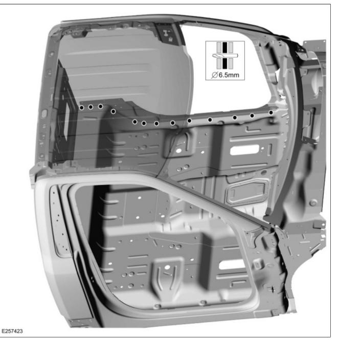
6. NOTE: Blind rivet or solid rivet fasteners may be used in place of <u>SPR</u> fasteners after enlarging holes to 6.5 mm.
