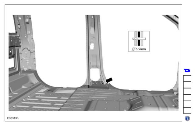
6. NOTE: <u>SPR</u> fasteners may not be placed directly over original <u>SPR</u> location. They must be placed adjacent to original location matching original quantity.
