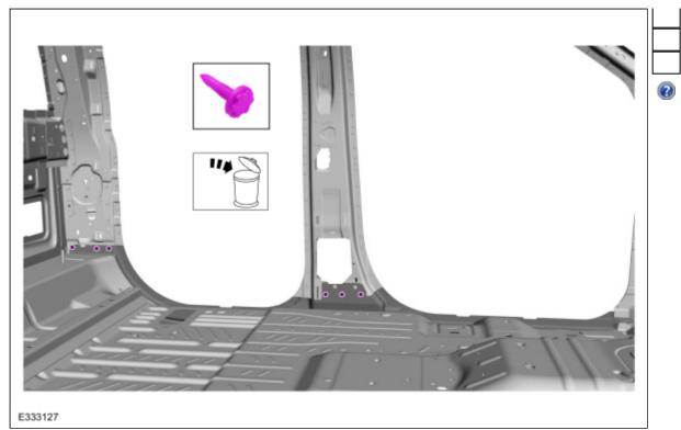
18. Remove and discard the A-pillar <u>FDS</u> fasteners. Use the General Equipment: Polydrive Bit Socket
