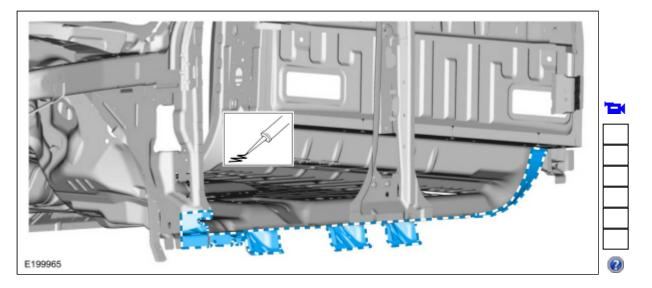
4. Install the rocker panel and clamp in position. Use the General Equipment: Locking Pliers
