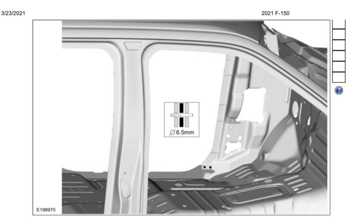
8. NOTE: <u>SPR</u> fasteners may not be placed directly over original <u>SPR</u> location. They must be placed adjacent to original location matching original quantity.
