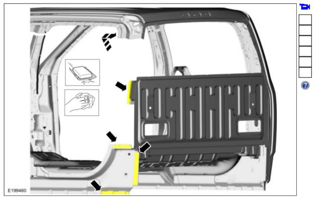
26. Sand using 80 grit sand paper to remove old adhesive and e-coat and clean.
