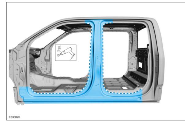
12. Remove and discard the B-pillar reinforcement <u>FDS</u> fasteners. Use the General Equipment: Polydrive Bit Socket
