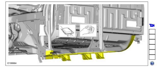
2. Sand using 80 grit sand paper to remove old adhesive and e-coat and clean.
