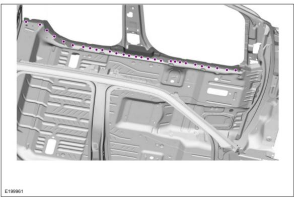
21. Remove the outer <u>SPR</u> fasteners. Use the General Equipment: Self-Piercing Rivet (SPR) Remover/Installer Use the General Equipment: Belt Sander
