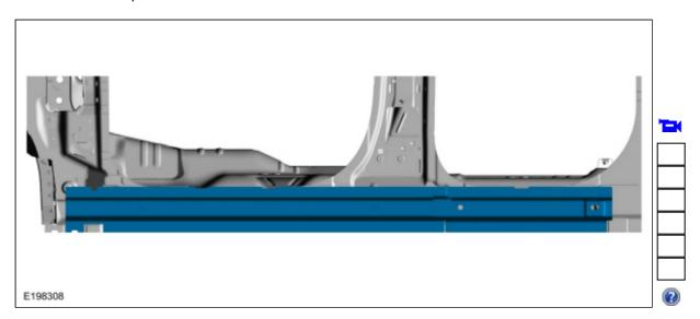
17. Remove and discard the B and C-pillar <u>FDS</u> fasteners. Use the General Equipment: Polydrive Bit Socket
