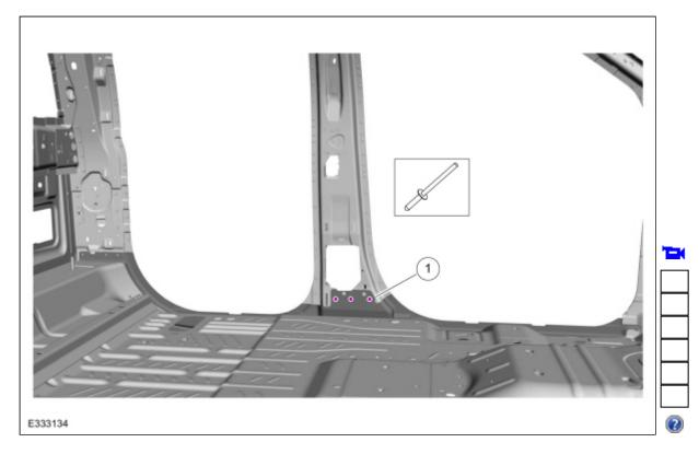
7. Drill 6.5 mm holes for fasteners. Use the General Equipment: 6.5 mm Drill Bit
