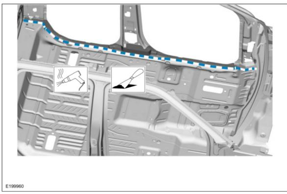
20. Remove and discard the floor pan-to-rocker panel <u>SPR</u> fasteners. Use the General Equipment: Self-Piercing Rivet (SPR) Remover/Installer Use the General Equipment: Belt Sander
