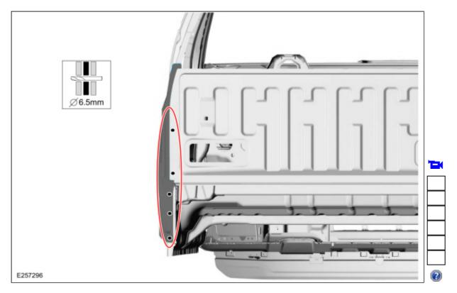
46. NOTE: <u>SPR</u> fasteners may not be placed directly over original <u>SPR</u> location. They must be placed adjacent to original location matching original quantity.
