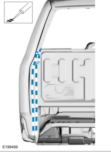
52. Seam Sealing: All seams must be sealed to production level. *Material*: Seam Sealer / TA-2-B, 3M™ 08308, LORD Fusor® 803DTM
