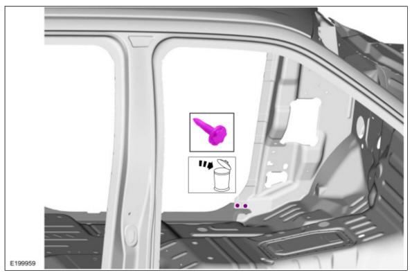
Remove the floor pan-to-rocker panel seam sealer.
