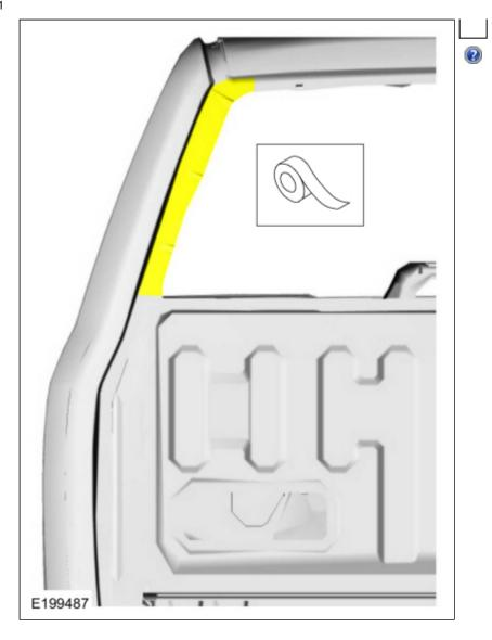
51. Seam Sealing: All seams must be sealed to production level. *Material*: Seam Sealer / TA-2-B, 3M<sup>™</sup> 08308, LORD Fusor® 803DTM
