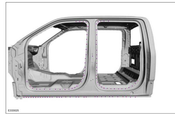
10. Measure and cut **the outer panel only** of the body side panel. Use the General Equipment: Air Body Saw Use the General Equipment: Spherical Cutter
