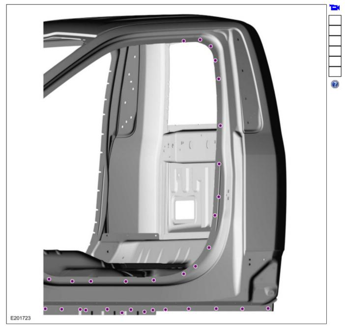
10. Remove the cab back seam sealer. Use the General Equipment: Scraper for Straight Edges Use the General Equipment: Hot Air Gun
