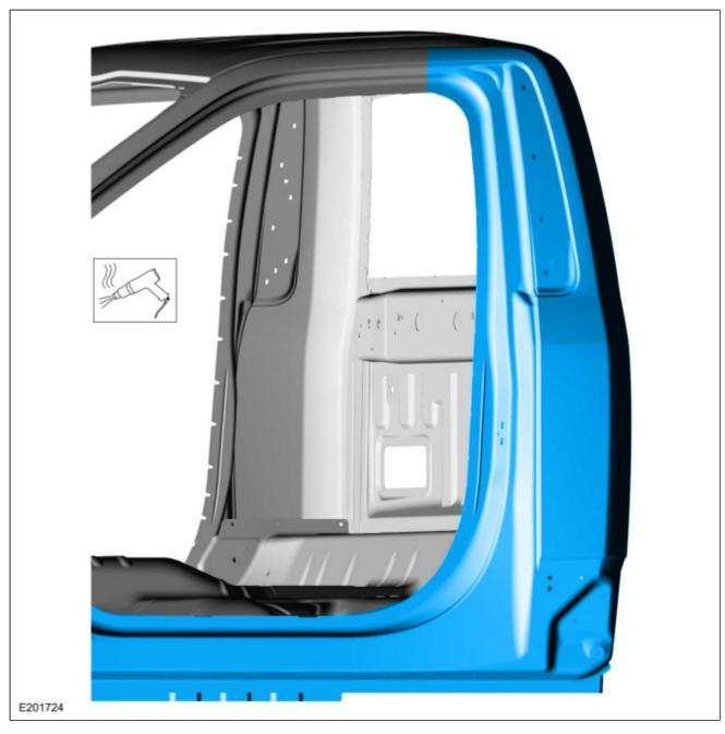
13. Remove and discard the <u>FDS</u> fasteners.
