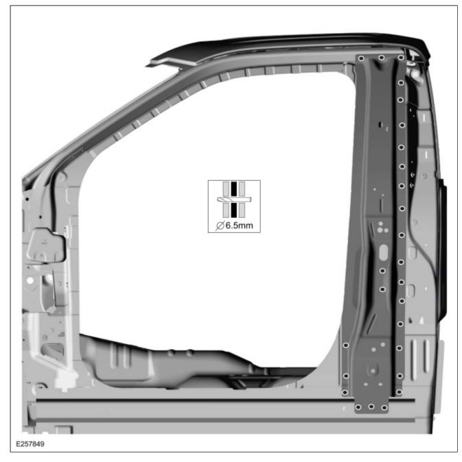
19. Install blind rivet fasteners.
