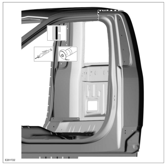
9. Remove the <u>SPR</u> fasteners.
