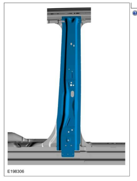
15. Remove the <u>SPR</u> fasteners in the rocker panel inner reinforcement.
