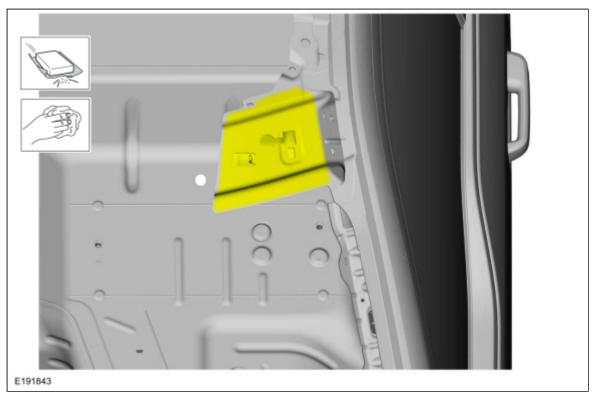
2. Sand the roof front frame using 80 grit sandpaper to remove e-coat and clean.
