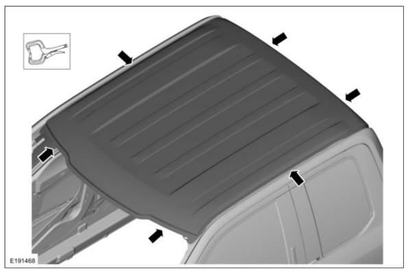
11. **NOTE:** <u>SPR</u> fasteners may not be placed directly over original <u>SPR</u> location. They must be placed adjacent to original location matching original quantity. **NOTE:** Solid rivets may be used in place of <u>SPR</u> in the original <u>SPR</u> location after enlarging hole to 6.5 mm.
