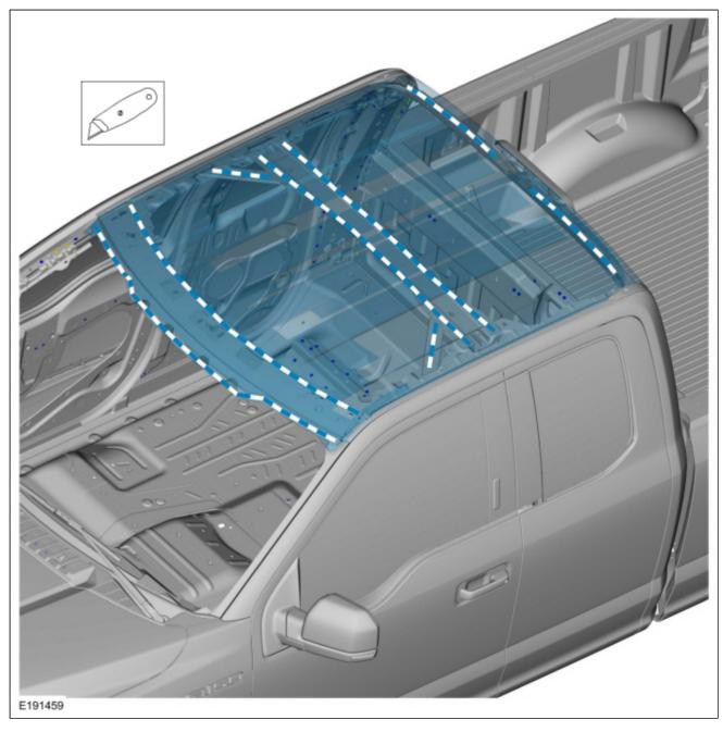
14. Separate the roof outer panel from the rear header panel. Use the General Equipment: Knife
