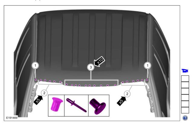
12. **NOTE:** <u>SPR</u> fasteners may not be placed directly over original <u>SPR</u> location. They must be placed adjacent to original location matching original quantity.
