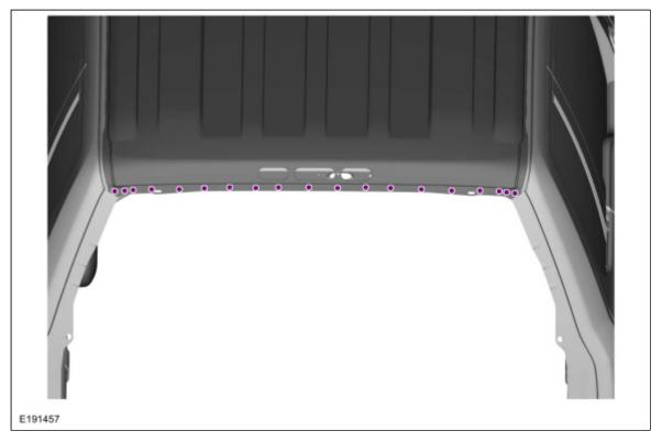
12. Carefully cut the **roof outer panel** only in the area shown (inboard on the roof ditch). Both sides. Use the General Equipment: Air Body Saw Use the General Equipment: Spherical Cutter
