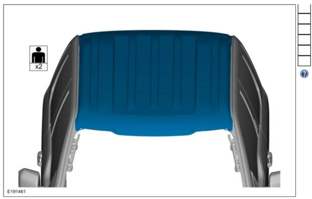
9. **NOTE:** Do not lift the roof panel to align to index marks. Slide the panel in position to reduce the possibility of breaking the adhesive bond.
