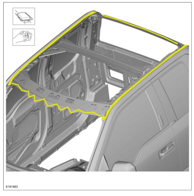
3. Sand to remove the e-coat and clean the roof panel mating surface using 80 grit sandpaper.
