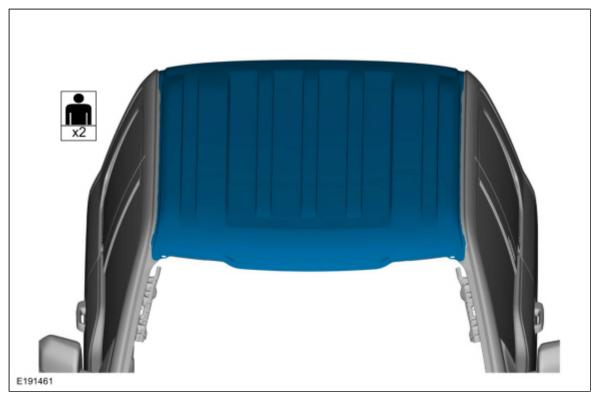
7. Apply adhesive to the roof bows, front header, rear header and roof ditch area mating surfaces. *Material*: Metal Bonding Adhesive / TA-1, TA-1-B, 3M™ 08115, LORD Fusor® 108B
