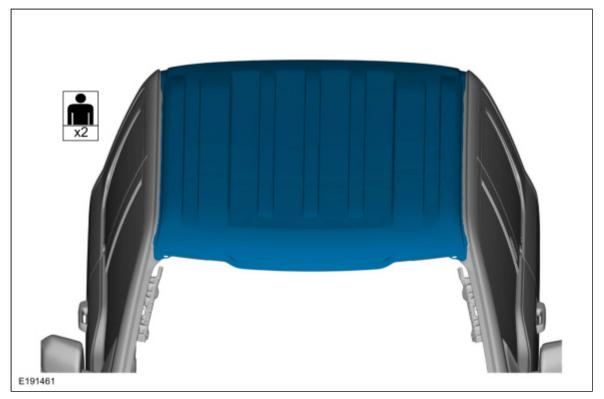
16. NOTE: Carefully grind the area smooth removing remaining portions of the factory laser weld. use caution to avoid thinning of the metal.
