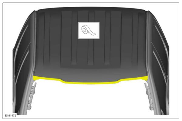
16. Apply roof ditch sealer following manufacturer's directions. *Material*: Roof Ditch Sealer / 3M™ 08307, LORD Fusor® 129
