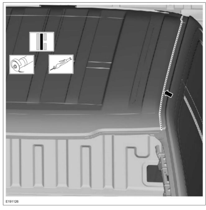
13. Leave as much foam as possible intact on the roof bows. Use the General Equipment: Knife
