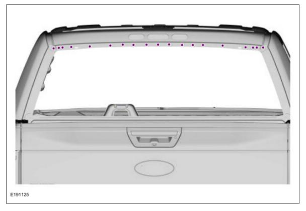
12. Carefully cut the roof **outer panel only** in the area shown (inboard on the roof ditch). Use the General Equipment: Air Body Saw Use the General Equipment: Spherical Cutter
