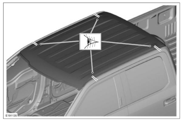
10. **NOTE**: Do not remove excess adhesive squeeze-out in the roof ditch area, smooth in to the joint to act as additional sealer.
