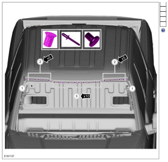
12. **NOTE**: <u>SPR</u> fasteners may not be placed directly over original <u>SPR</u> location. They must be placed adjacent to original location matching original quantity. **NOTE**: Blind or solid rivets may be used in place of <u>SPR</u> in the original <u>SPR</u> location after enlarging hole to 6.5 mm.
