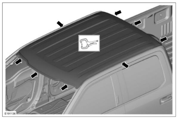
11. **NOTE:** <u>SPR</u> fasteners may not be placed directly over original <u>SPR</u> location. They must be placed adjacent to original location matching original quantity. **NOTE:** Blind or solid rivets may be used in place of <u>SPR</u> in the original <u>SPR</u> location after enlarging hole to 6.5 mm.
