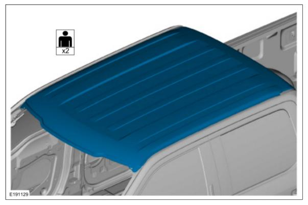
7. Apply adhesive to the roof bows, front header panel, rear header panel and roof ditch mating surfaces. *Material*: Metal Bonding Adhesive / TA-1, TA-1-B, 3M™ 08115, LORD Fusor® 108B
