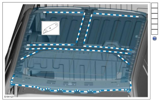
14. Separate the roof outer panel from the rear header panel. Use the General Equipment: Knife
