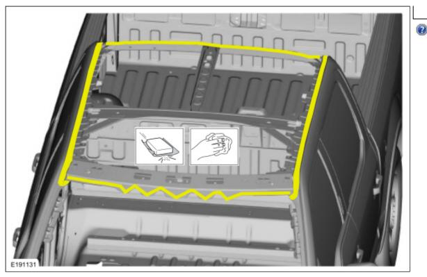
3. Sand to remove the e-coat and clean the roof panel mating surface using 80 grit sandpaper.
