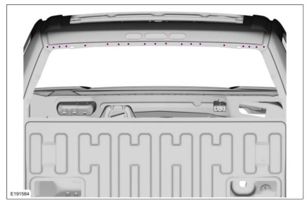
13. Carefully cut the roof **outer panel only** in the area shown (inboard on the roof ditch, both sides). Use the General Equipment: Air Body Saw Use the General Equipment: Spherical Cutter
