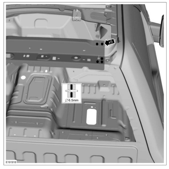
6. **NOTE:** <u>SPR</u> fasteners may not be placed directly over original <u>SPR</u> location. They must be placed adjacent to original location matching original quantity. **NOTE:** Blind or solid rivets may be used in place of <u>SPR</u> in the original <u>SPR</u> location after enlarging hole to 6.5 mm.
