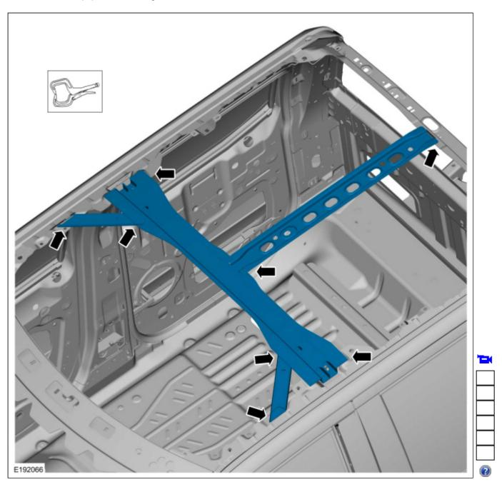
2. Drill 6.5 mm rivet holes as indicated.
