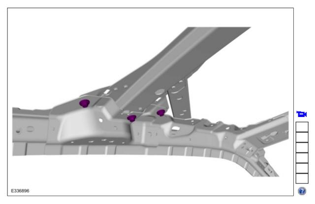
4. **NOTE:** <u>SPR</u> fasteners may not be placed directly over original <u>SPR</u> location. They must be placed adjacent to original location matching original quantity. **NOTE:** Solid rivets or blind fasteners may be used in place of <u>SPR</u> fasteners after enlarging the existing hole to 6.5 mm.
