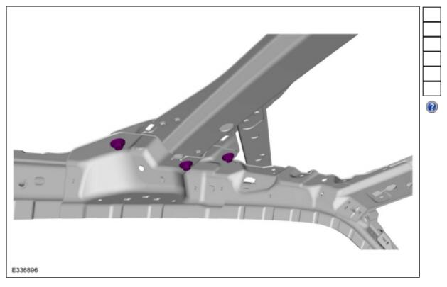
5. Remove the roof reinforcement.
