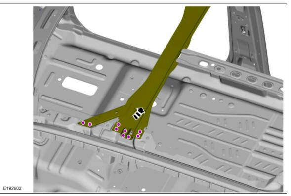
16. Remove the <u>SPR</u> fasteners, remove and discard the <u>FDS</u> fasteners and the B-pillar gusset from the roof side rail. Use the General Equipment: Self-Piercing Rivet (SPR) Remover/Installer Use the General Equipment: Belt Sander Use the General Equipment: Polydrive Bit Socket
