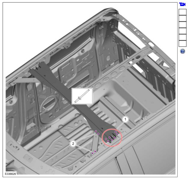
43. Position, clamp and drill as indicated. Use the General Equipment: Locking Pliers Use the General Equipment: 6.5 mm Drill Bit
