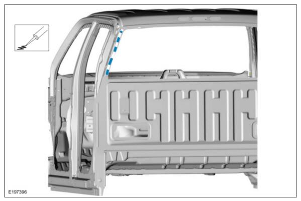
8. Install, align and clamp the service panel.
