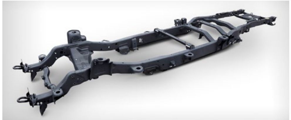
The 2017 Super Duty frame comes in several crossmember configurations, depending on wheelbase size.
