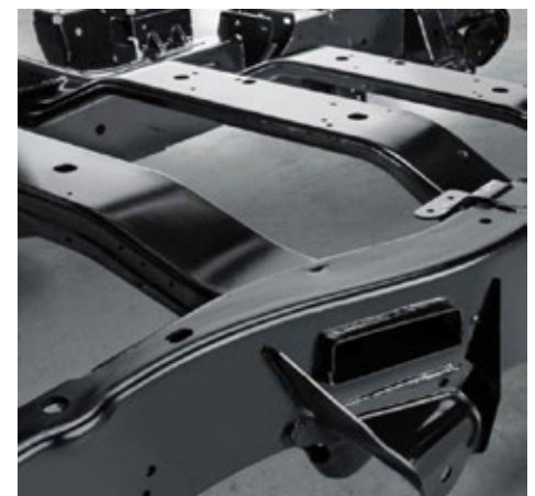
The welded-through crossmembers help make the frame 24 times stiffer than previous models.
