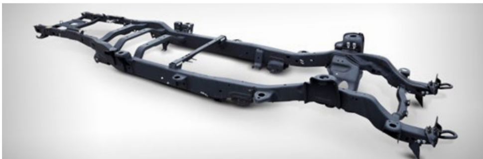
95 percent of the frame is made of high-strength steel, six times more than the previous frame.
