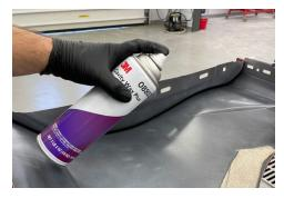
will require body filler, seam sealer or coatings. This is the only way to truly restore the factory-applied corrosion protection system. Remember the e-coat process mentioned previously? That is done at the factory before any gravel coatings, undercoating or sealers are applied and it is done without using direct-to-metal (DTM) products.
